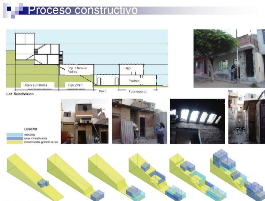
Figure 2. Gradual 25 year build out across the lot from single shack to consolidated multi-room dwelling with separate sections for 2-3 households (parents and son; future apartment for parents; daughter and family, etc.) Note the dilapidation associated with intensive use. (Courtesy of Susanna Rojas Williams.)
