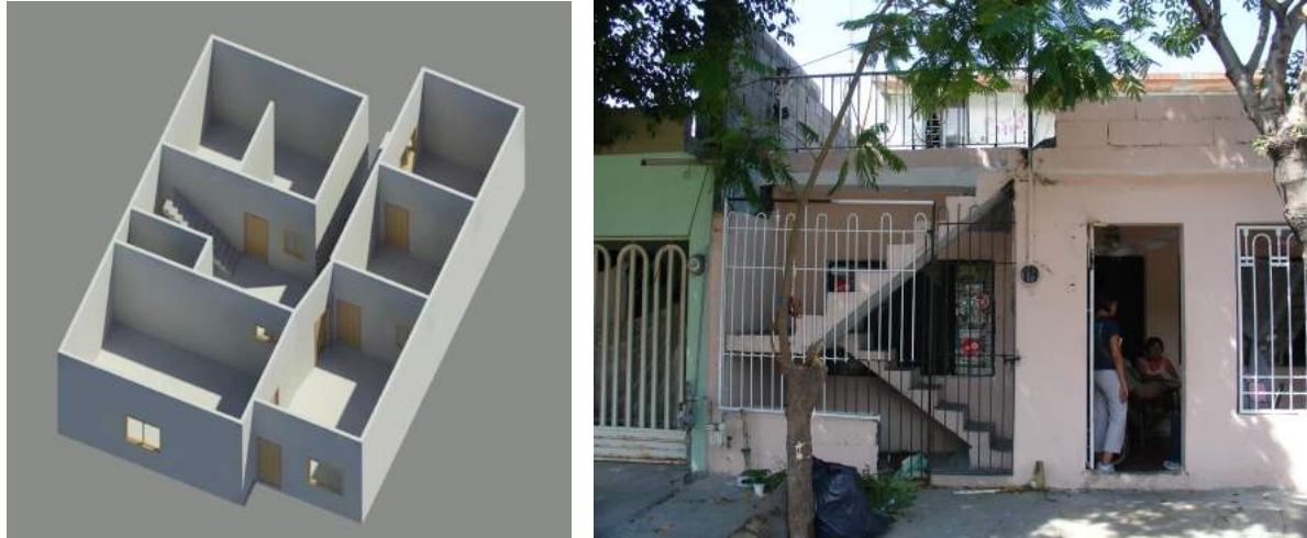
Figure 4.5a-b. Gradual build-out of one home in Valle Santa Lucía and how it can lead to poor or non-existent natural lighting in some rooms, and to “dead” (unusable spaces) below stairs (photo)
