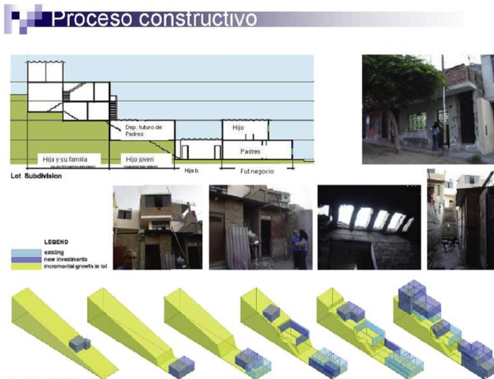
Fig. 2. Gradual 25 year build out across the lot from single shack to consolidated multi-room dwelling with separate sections for 2–3 households (parents and son; future apartment for parents; daughter and family, etc.) Note the dilapidation associated with intensive use. (Courtesy of Susanna Rojas Williams.)
