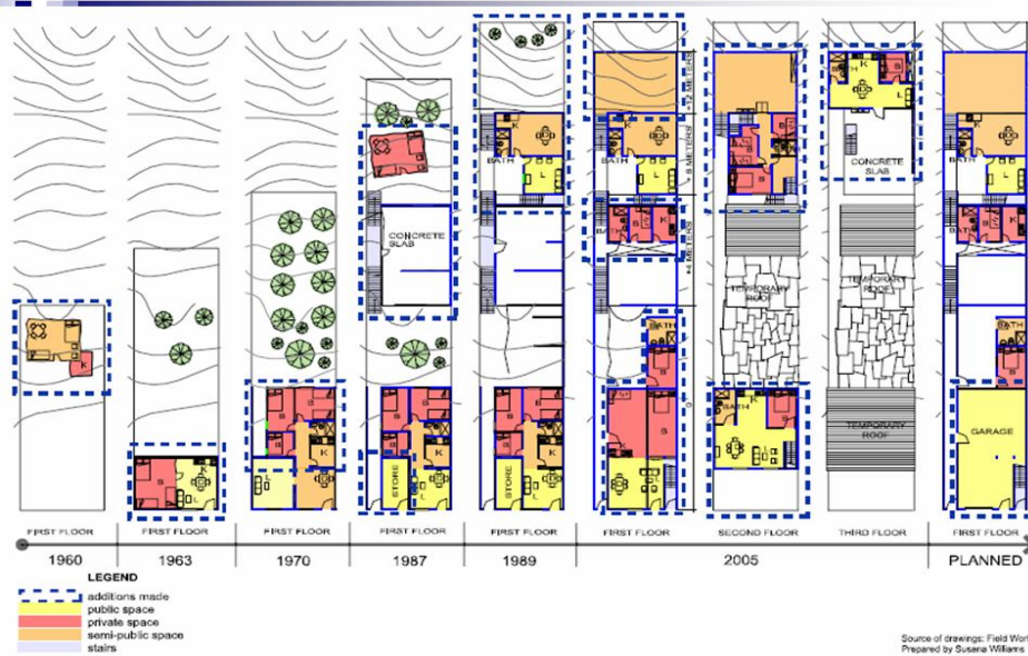
Figure 1a. Sketch plan of the physical development of a squatter dwelling, Lima
